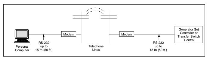
Figure 2-14 Remote Single Connection
